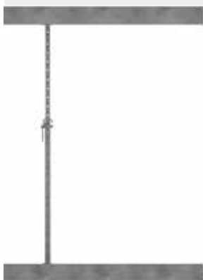
Cotter pin in working position
